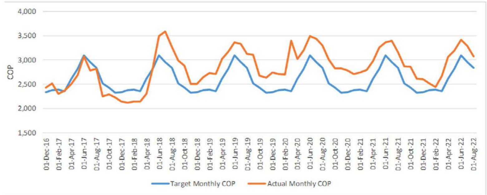
A lifetime trend view of the COP of a medium-sized supermarket refrigeration system (target vs actual). Note the annual variations due to changing ambient conditions, as well as the increase in actual COP approximately 15 months after implementing a modification aimed at increasing the COP.
