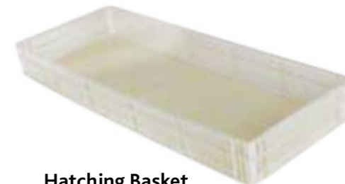
Hatching Basket Size: 976 x 388 x 116 mm (H) Carrying Load: 20 kg Max Load on Base: 160 kg Stack Height: 105 mm Material: Polypropylene
